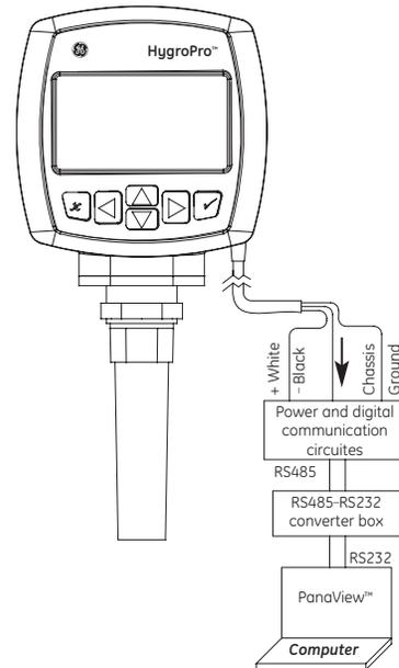
*Digital communications wiring connection
